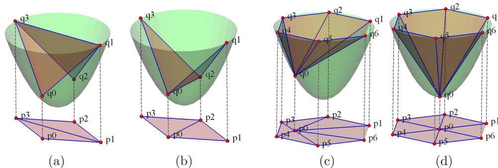
Figure 1: Illustration of minimizing interpolation error in two ways: edge swapping (a-b) and vertex-repositioning (c-d). The mesh quality in (b) is improved by swapping the edges but keeping the vertices fixed. The interpolation error can also be reduced (hence mesh quality is improved) by moving the vertex  $p_0$  in (c) to a new position in (d), where the edge connections are kept unchanged.
