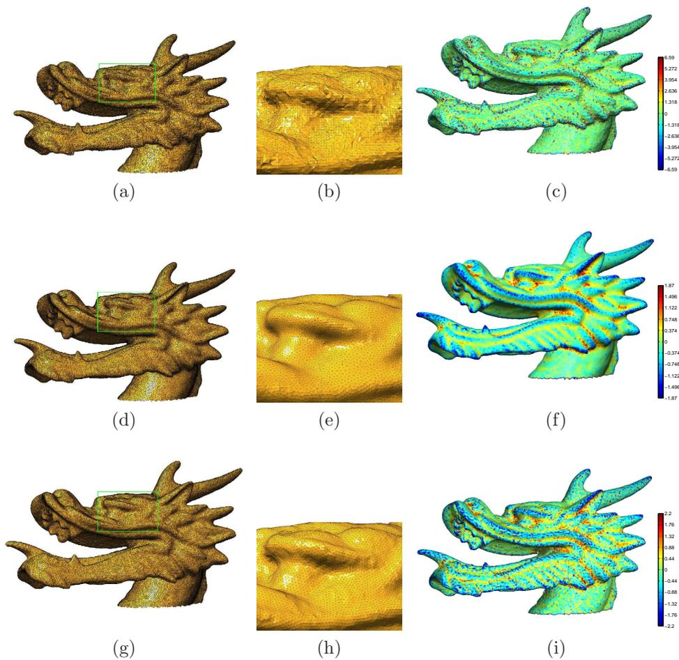
Figure 8: Mesh smoothing of the dragon head model. (a-c) Original mesh with noise and extremely low quality (mesh courtesy of Stanford University - 3D scanning repository). (d-f) Smoothed mesh with significantly improved quality. (g-i) Remeshed results using [17].
