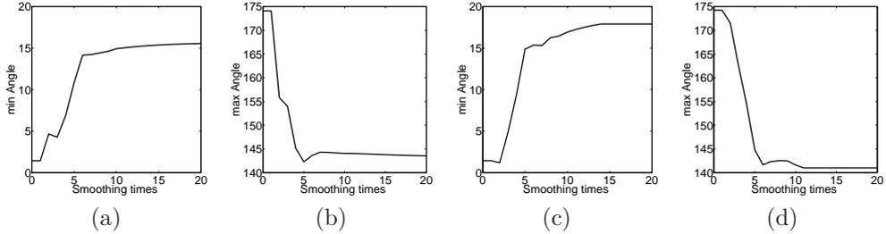
Figure 4: The convergence of Algorithm 1. (a-b) show how the minimal and maximal angles (in degrees) change with respect to the number of iterations applied to the bimba model. (c-d) show how the minimal and maximal angles (in degrees) change with respect to the number of iterations applied to the elephant model.
