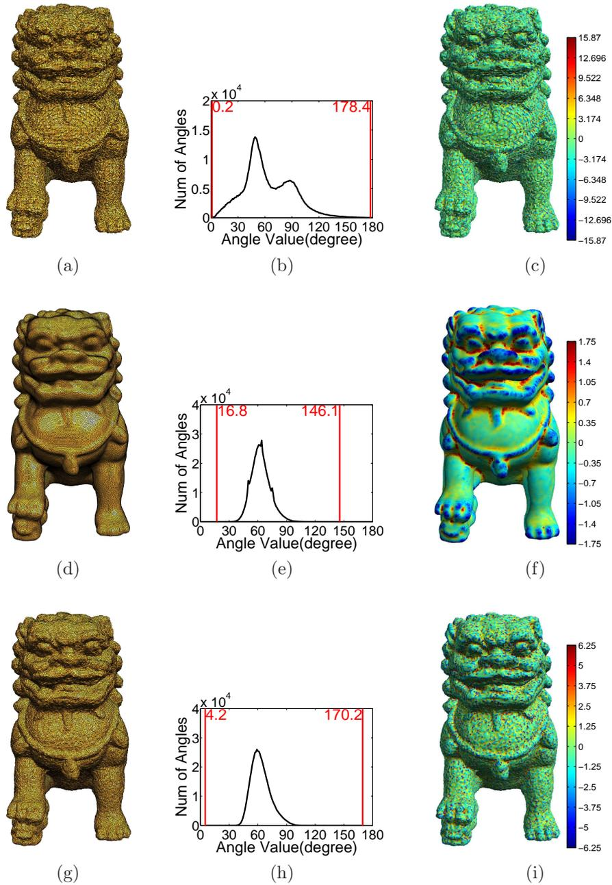
Figure 9: Illustration of the feature-preserving and noise-removing S-ODT method (Algorithm 3) and comparison with remeshing method in [18]. The original and smoothed meshes of the Chinese lion are shown on the top and middle respectively. The remeshed mesh is shown on the bottom. The model is provided courtesy of INRIA by the [AIM@SHAPE](mailto:AIM@SHAPE) Shape Repository.
