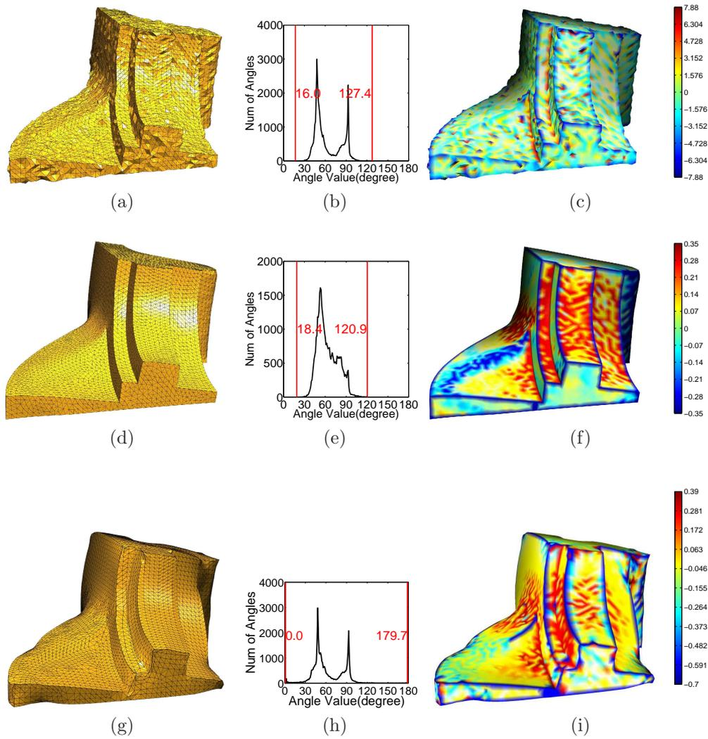
Figure 10: Illustration of the feature-preserving and noise-removing S-ODT method (Algorithm 3). The original and smoothed meshes of the fan disk and their corresponding histograms and curvature maps are shown on the top and middle rows respectively. And the bilateral filtering [10] result is shown in the bottom row.
