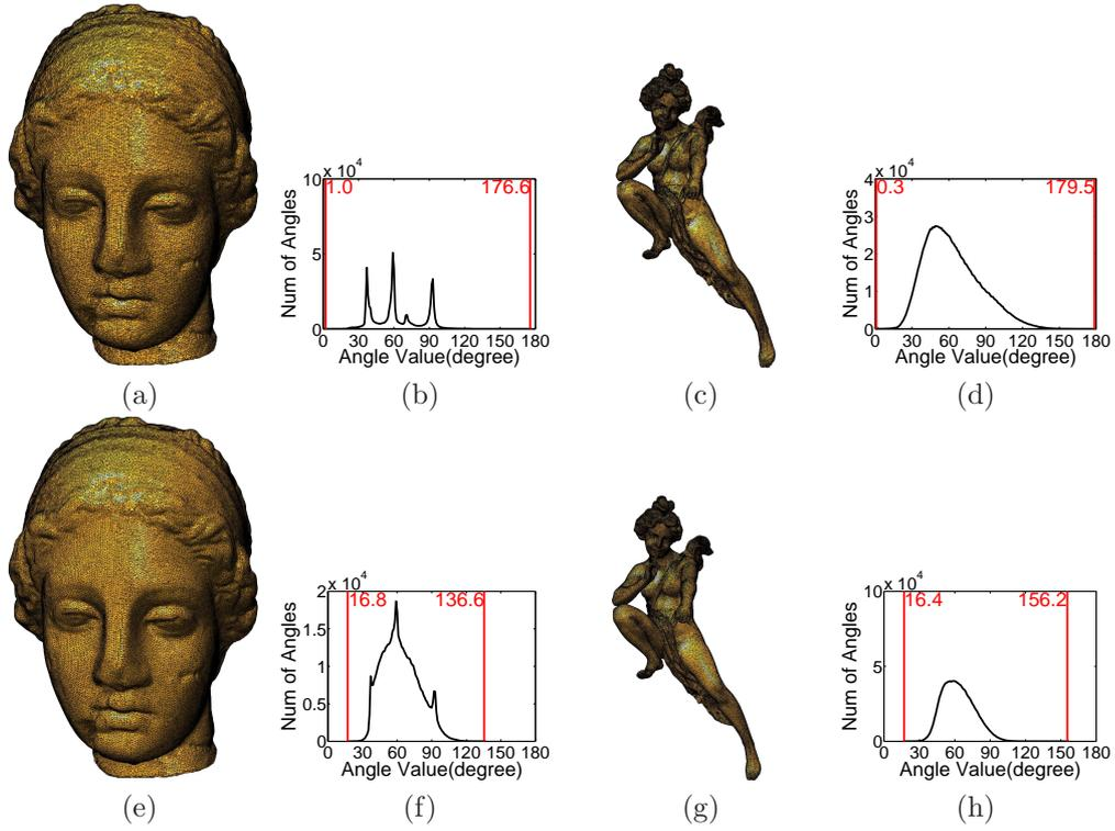
Figure 11: Illustration of the mesh quality improvement of S-ODT method (Algorithm 3) on the Venus and Angel models.
