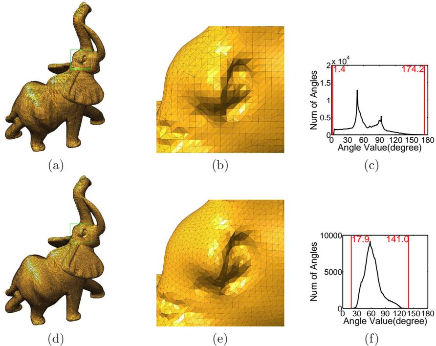
Figure 3: The elephant mesh model. (a-c) show the original surface mesh, a closer view and the angle histogram of the mesh. (d-f) show the smoothed mesh and the corresponding histogram after applying the S-ODT (Algorithm 1) 20 times. The minimum and maximum angles in both meshes are indicated in red in the histograms. The model is provided courtesy of INRIA by the AIM@SHAPE Shape Repository.
