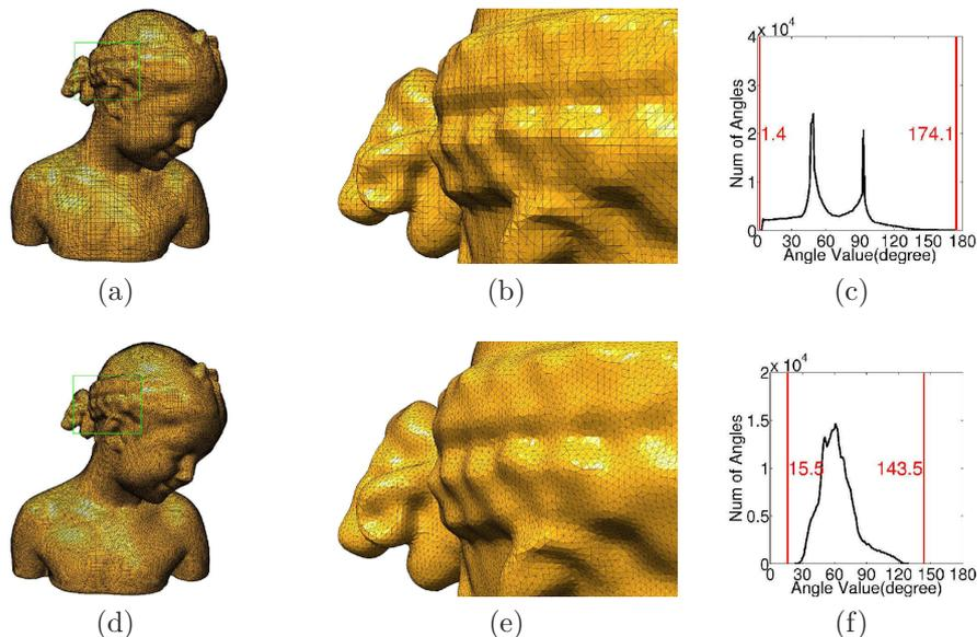
Figure 2: The bimba mesh model. (a-c) show the original surface mesh, a closer view and the angle histogram of the mesh. (d-f) show the smoothed mesh and the corresponding histogram after applying the S-ODT (Algorithm 1) 20 times. The minimum and maximum angles in both meshes are indicated in red in the histograms. The original model is provided courtesy of IMATI and INRIA by the AIM@SHAPE Shape Repository.
