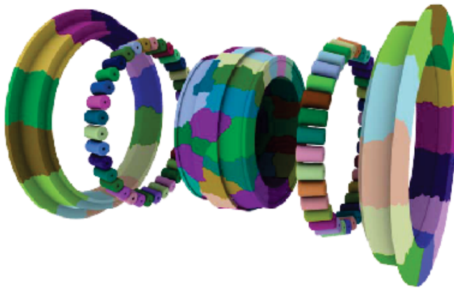
Figure 1. Roller bearings of wind generator
