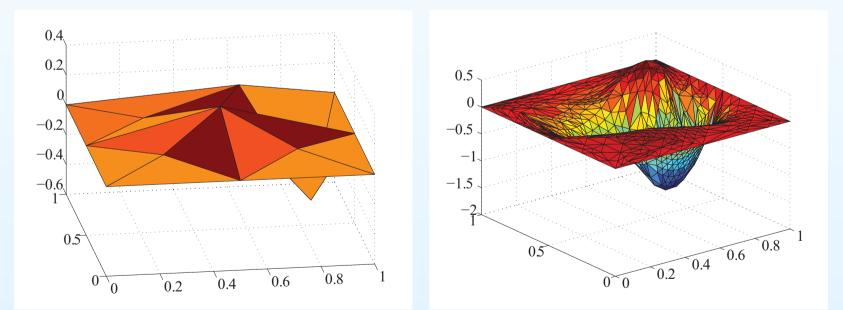
$U_1$  on a coarse mesh and the total error of  $U_2$ Independently adapting each component mesh makes the error worse!
