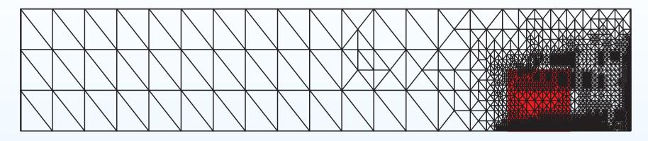
Final Mesh for an Average Error in a Patch (3,500 Elements)
