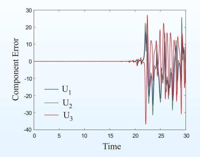
Componentwise "Errors" Computed using Solutions with Tolerances .001 and .0001
