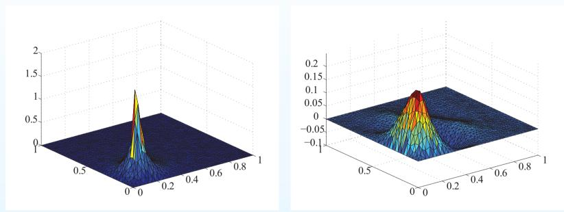
Primary and decomposition-contribution adjoint solutions The adjoint solution for the functional on  $u_2$  is large due to the adjoint data (an approximate delta function). The adjoint associated with the information transferred between the components is large in the same region. This indicates that the accuracy of  $u_1$  in this region impacts the accuracy of  $u_2$ .
