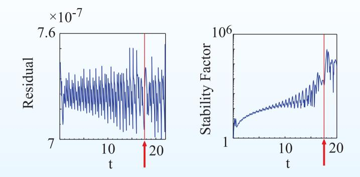
The Residual and Stability Factor for the Inaccurate Solution The residual is small even when the error is large. In fact, this is a theorem: the residual of a consistent discretization for a wide class of problems is small regardless of the size of the error! This indicates the problems in trying to use the residual or "local error" for adaptive error control. On the other hand, the size of the adjoint grows at an exponential rate during a brief period at the time when the error becomes 100%.
